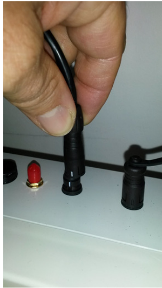
a) Connect the optical tube to the computer
