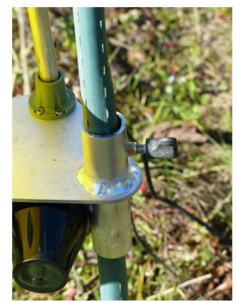
e) A 16mm diam. post can help adapt the height of the trap.
