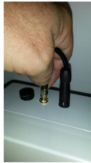
b) Connect the antenna to the computer
