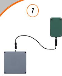
Connect the Battery Pack to the Camera
