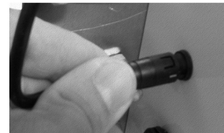
g) Connect the Camera cable to the grey box 4-pins connector
