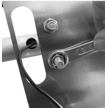
c) Tighten the fixing bolts.
